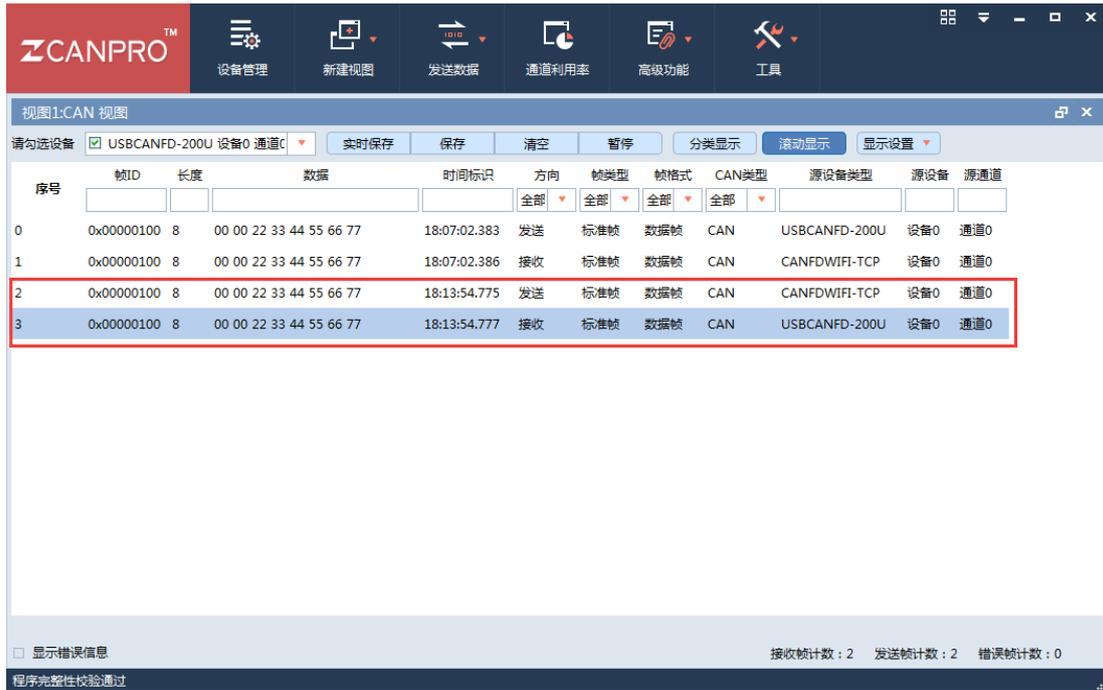
Figure 5.22 CANFDWIFI-TCP send result
