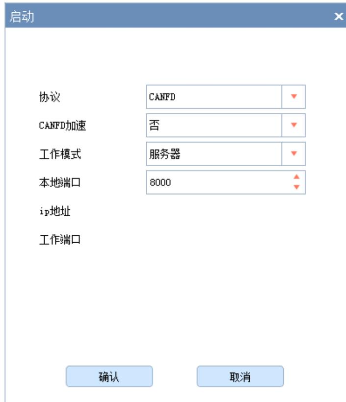
Figure 5.29 Starting the CANFDNET-TCP server
