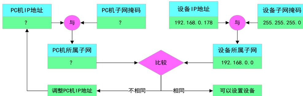
Figure 5.6 Detection process on the same network segment
