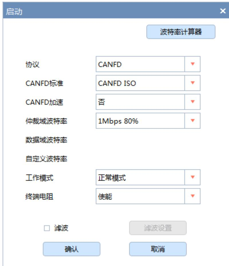
Figure 5.11 Default startup parameters of USBCANFD-200U
