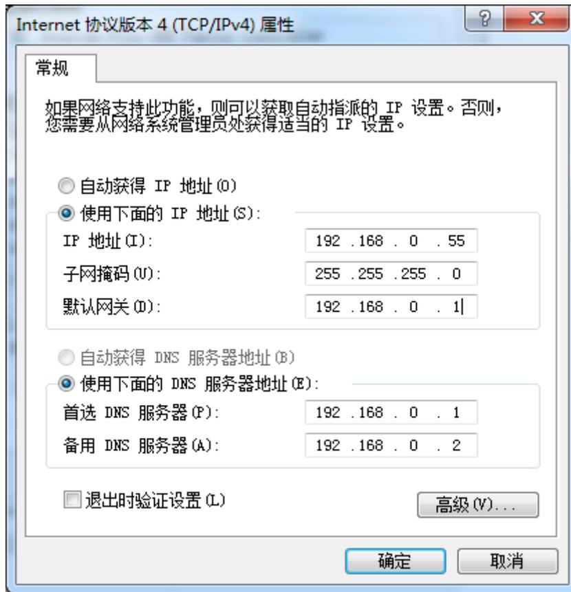
Figure 5.7 TCP/IP properties
