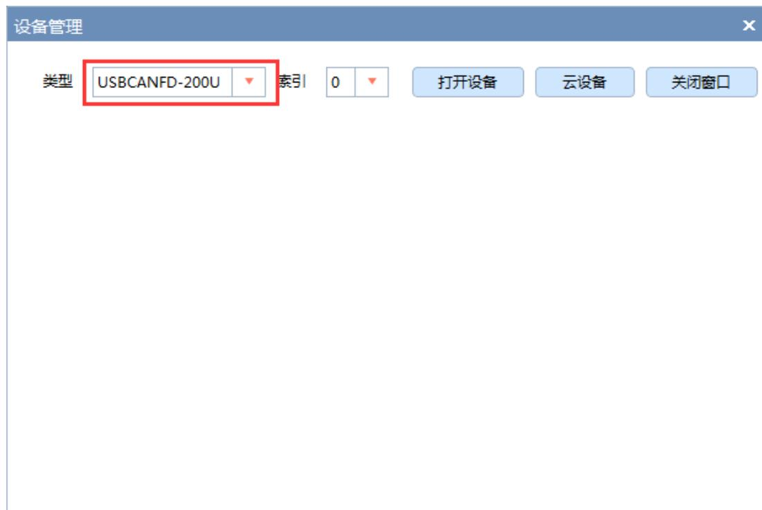
Figure 5.9 Starting ZCANPRO and selecting the USBCANFD-200U
