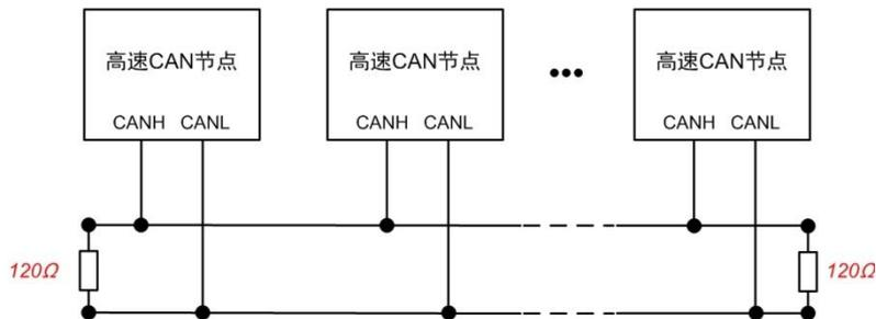
Figure 4.2 Typical high-speed CAN network connection
