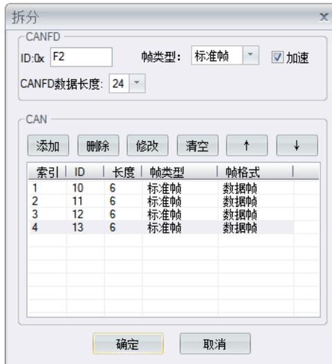
Figure 4.38 24-byte CANFD split into 4 6-byte CAN settings
