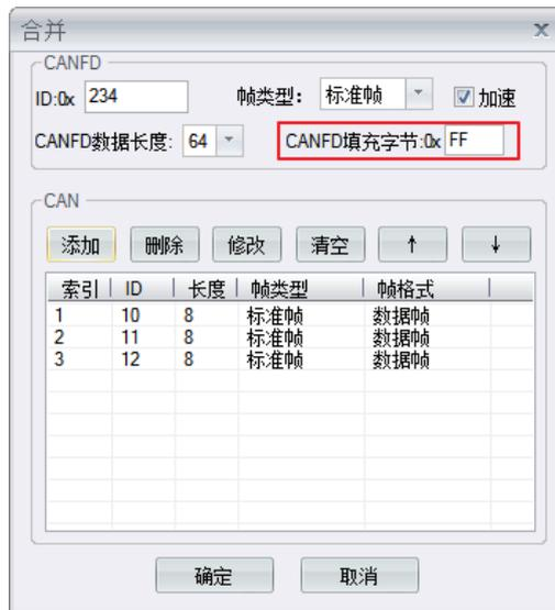
Figure 4.32 Total length of combined CAN less than CANFD
