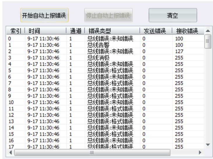
The screenshot shows a software interface for reporting CAN errors. At the top, there are three buttons: '开始自动上报错误' (Start automatic error reporting), '停止自动上报错误' (Stop automatic error reporting), and '清空' (Clear). Below these buttons is a table with the following data:
