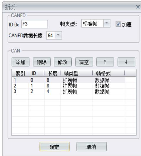
Figure 4.40 64-byte CANFD split into two 8-byte CAN settings
