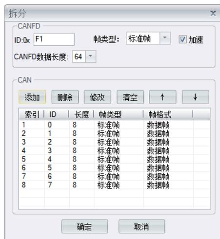
Figure 4.36 64-byte CANFD split into eight 8-byte CAN settings
