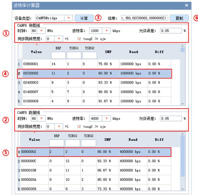
Figure 4.8 Using the baud rate calculator
