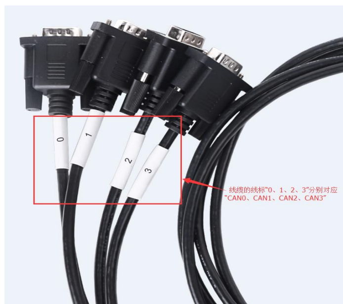
Figure 2.2 DB37 to 4xDB9 cable channel identification
